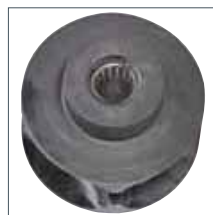
Load chain sheave with needle bearing
