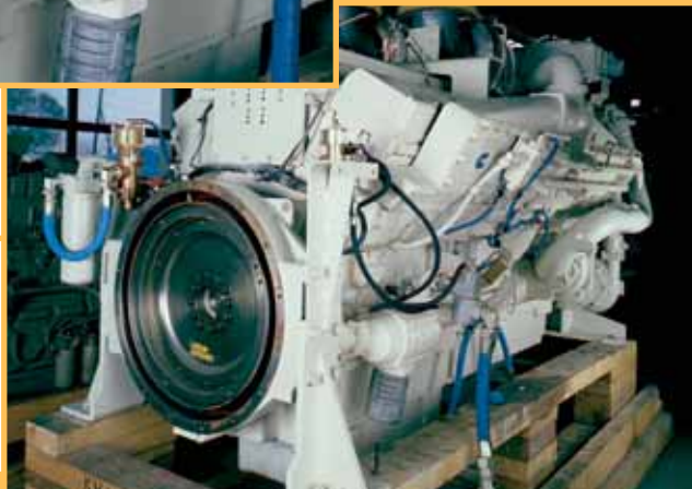
The SS815GB03R31 starter is shown mounted on a Cummins KTA50-M2 piped with the IR SRV150 Relay Valve.
