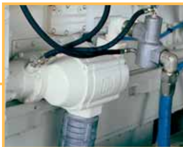
The SS815GB03R31 starter is shown mounted on a Cummins KTA50-M2 piped with the IR SRV150 Relay Valve.
