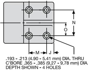
.193 - .213 (4.90 - 5.41 mm) DIA. THRU C'BORE .365 - .385 (9.27 - 9.78 mm) DIA. X .193 - .213 DEEP (FOR Y154-51 SCREWS)
