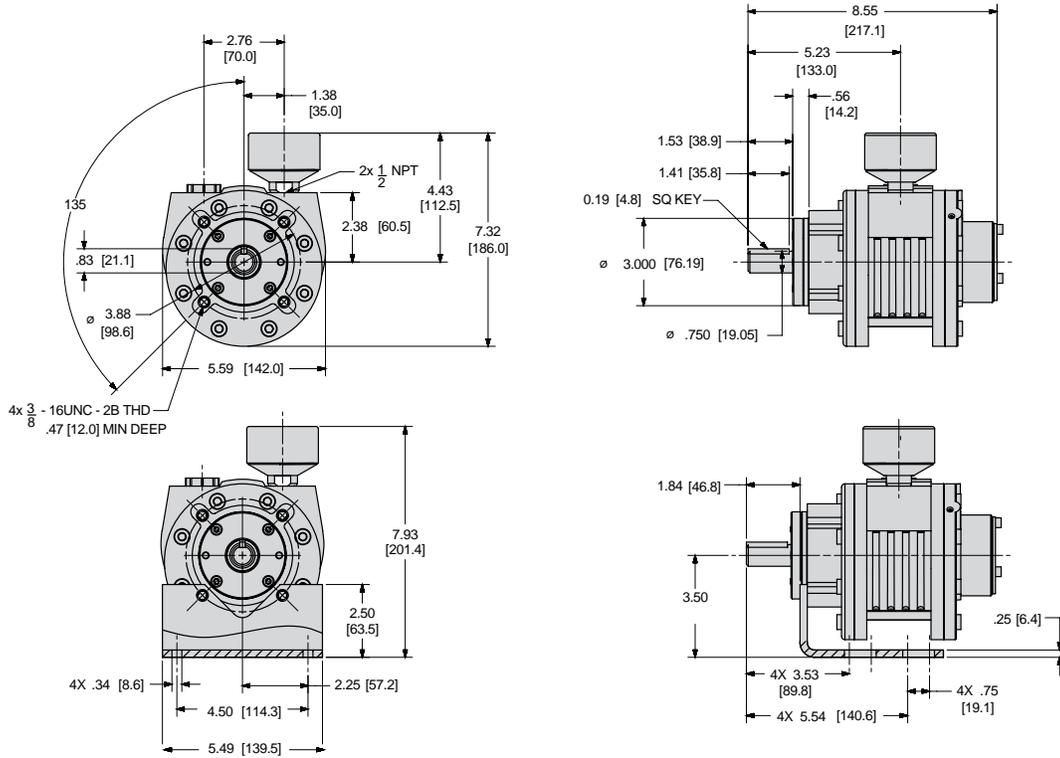
**SM8AMAN Lube Free Multi-Vane Air Motors NEMA Mount Dimensions**
