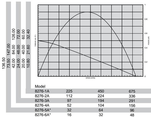
\*NOTE: Maximum torque recommended for planetary gear system on these models requires shear key with 150 ft./lbs. shear strength.
