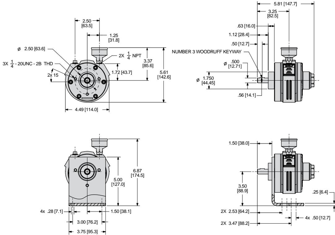
**SM4AMAN Lube Free Multi-Vane Air Motors NEMA Mount Dimensions**
