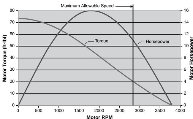
Figure 2: MMP150 Air Motor Performance
