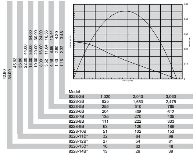
\*\*NOTE: Maximum torque recommended for planetary gear system on these models requires shear key with 60 ft./lbs. shear strength.
