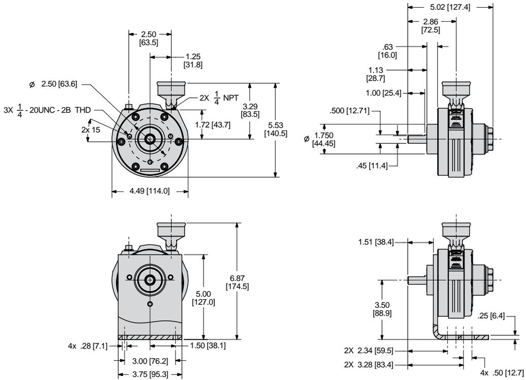
**SM2AMAN Lube Free Multi-Vane Air Motors NEMA Mount Dimensions**
