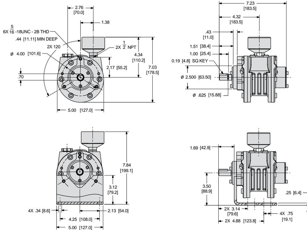
**SM6AMAN Lube Free Multi-Vane Air Motors NEMA Mount Dimensions**
