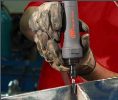
Weld cleaning and smoothing
