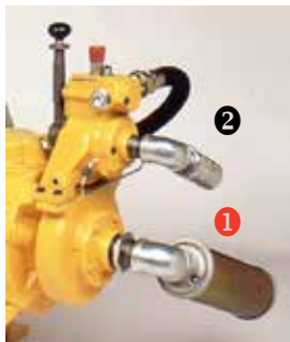
Control Exhaust (top) and Motor Exhaust (bottom)
