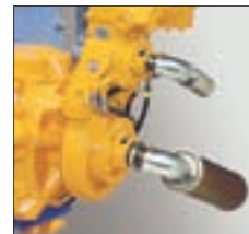
Exhaust mufflers (option J5)
