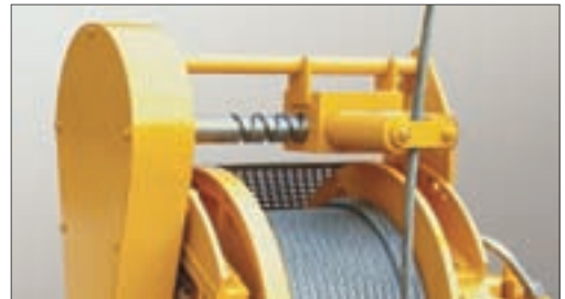
Spooling device on LS5000R
