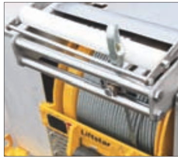
Automatic spooling device
