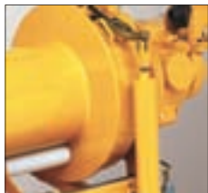
Automatic drum brake
