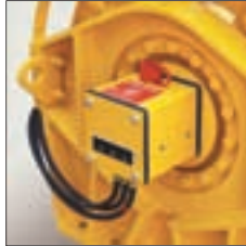
Limit switches on LS5000R
