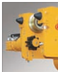
Rack & pinion drive
