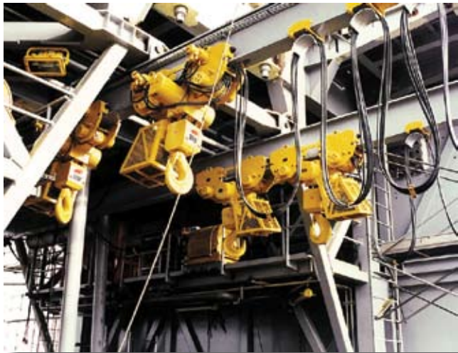
BS75LCH3 (2 x 75-ton) hydraulic systems used on a rig
