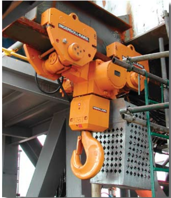
BS75LCA3 (75-ton) air system – 1 hoist shown
