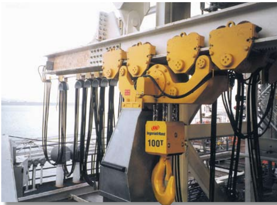
Liftchain 200-ton BOP Handling System (1 hoist shown)
