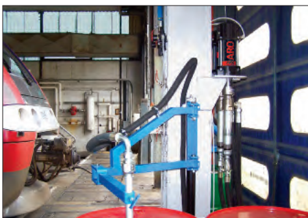
2-ball piston pump 9:1 ratio, used in a customised lubrication process
