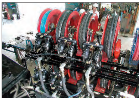
UL approved fuel pump 1" size, used assembled on skid dedicated in the aviation to fill and unload kerosene
