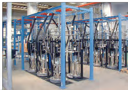
Large extrusion piston pumps, 13:1 ratio, installed on an offset ink formulation system process
